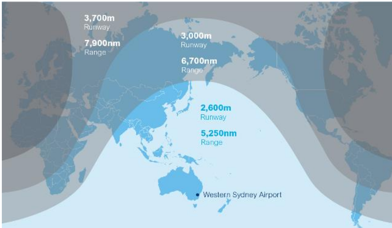
Figure 7: Boeing 777-300ER indicative range with maximum take-off weight
