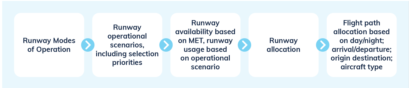
Figure 11.6 Process to allocate a WSI flight operation to a runway and flight path
